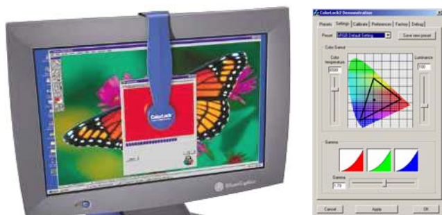
Figure 4. Sensor attached during measurement; "Settings" calibration window.
